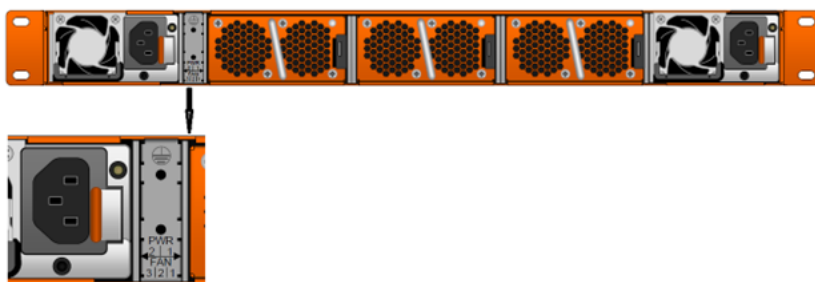
Figure 12 Holes for Ground Screws
